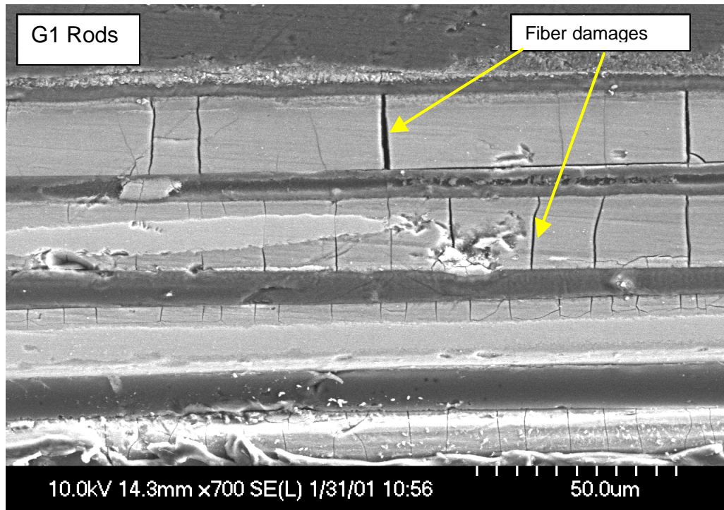
Figure 46: SEM longitudinal section of G1 specimens
