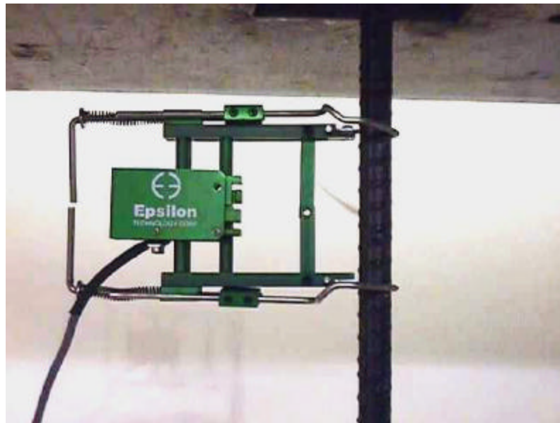
Figure 20: Extensometer mounted to the tensile specimen
