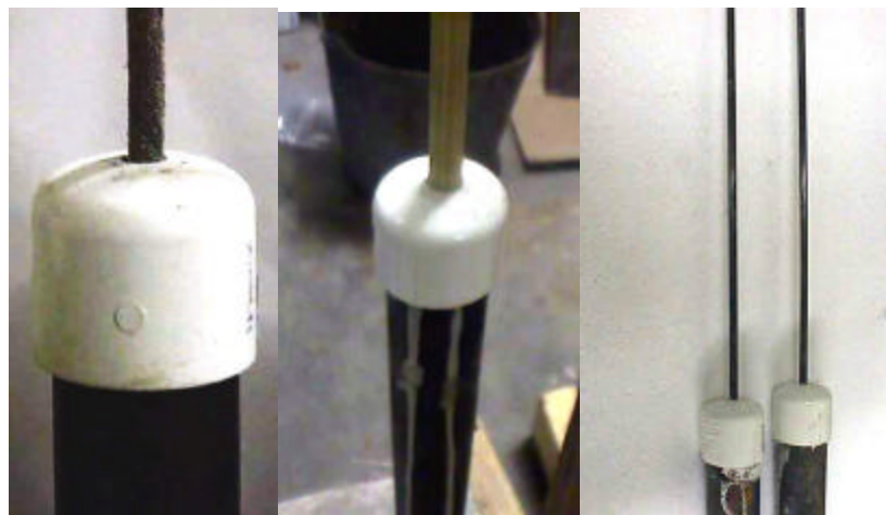
Figure 17: PVC drilled caps used for alignment
